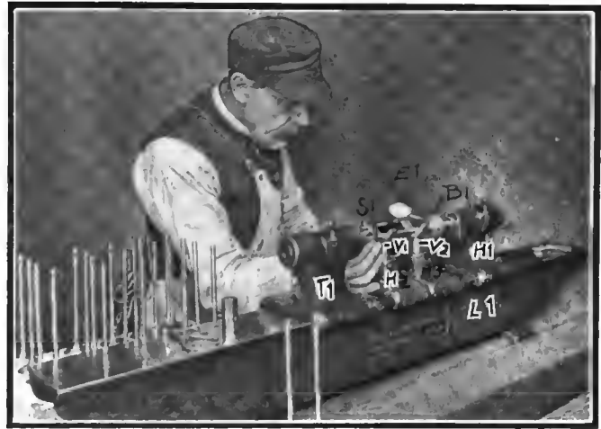
Fig. 9—Depicting the method in vogue in the Packard plant for inspecting valves
